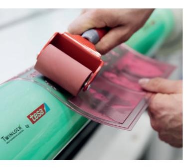
The concept of tesa Twinlock® is simple: a self-adhesive and compressible sleeve to mount your flexo printing plates.
