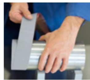
Keep on wrapping the roller with the tape at even angles, leaving no gaps in between the layers.
