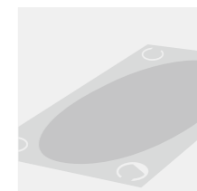
Temporary fixing aid, which keeps the cut out in place
