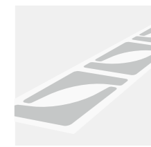
Die cuts interlaced to save material
