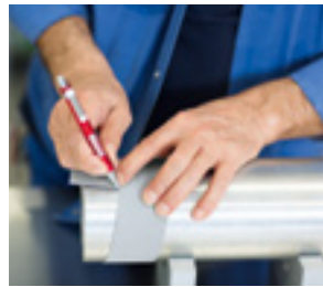
Wrap the tape once around the roller at the desired angle and mark the point where the end of the roll meets the second turn of the tape.
