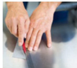
Put the tape on a flat surface and cut it diagonally from the end of the roll to the marked point of the tape.
