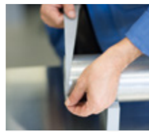
Remove the liner and start applying the tape, starting from the edge of the roller.
