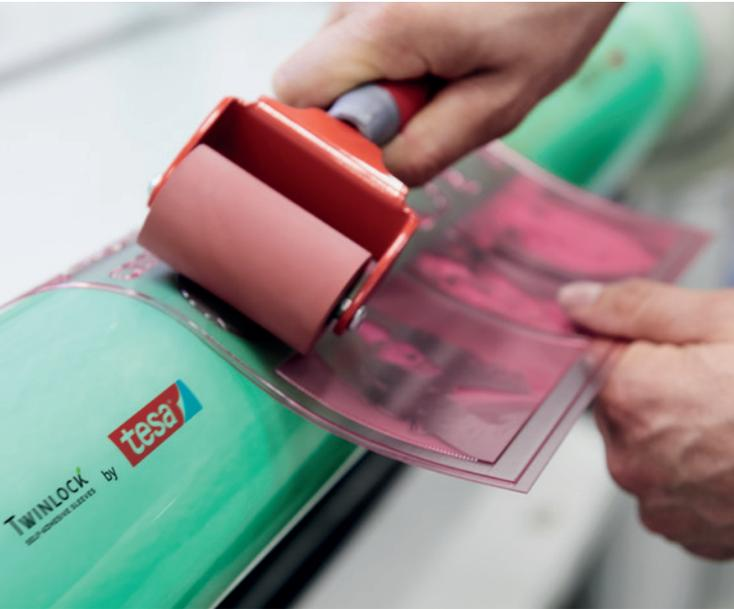
The concept of tesa Twinlock® is simple: a self-adhesive and compressible sleeve to mount your flexo printing plates.
