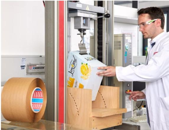
tesa® 51345 has been developed to reinforce critical stress areas like side hole handles, flap handles, and top hole handles. Tests have proven same level of performance strength as market standard film-based tapes.
