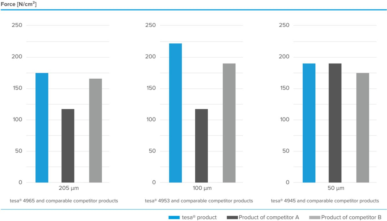
The dynamic shear test results highlight the exceptional performance of the three tesa® tapes under dynamic shear loads. The three compared 50 µm tape versions demonstrate comparable strength. While the products of competitor A fall short in dynamic shear resistance for their 200 µm and 100 µm tape versions. The products of competitor B show performance levels equal to tesa's offerings.
