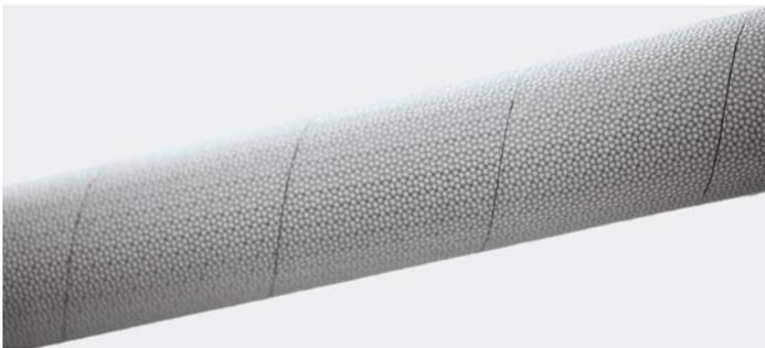
Complete roller spiral wrapped, providing grip and a non-stick surface.
