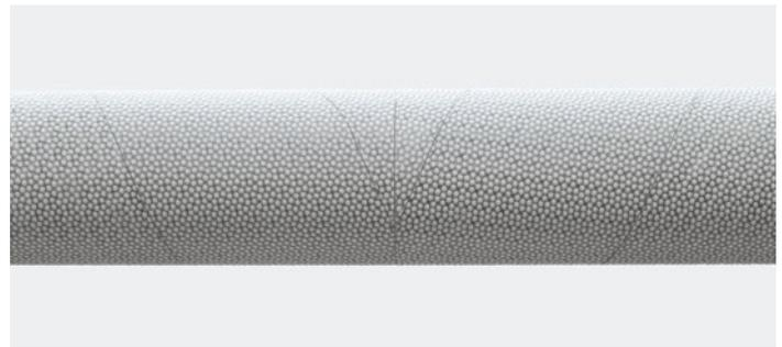
Other designs of wrapping are also possible. Starting from the middle and wrapping to the ends aids in pulling the material evenly across the roller to eliminate creases.
