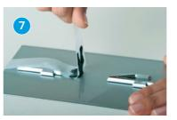
Immediately after bonding, peel off at a 90° angle. Large adhesive areas can be removed quickly by using this method
