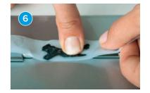
Ensure that the film is completely bonded to the adhesive residue by pressing it with your thumb. As the residue might be still hot, wear protective gloves.
