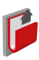
The test should be carried out as follows: Remove the liner from the tape and attach an aluminum foil strip to it. The aluminum strip should be at least the same width as the tape and overlap the tape on one end to create a hold.
