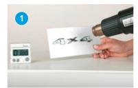
Heat up the part with an air blower to at least 80 to 100°C for minimum one minute.\*
