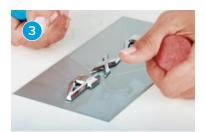
Position the fishing line between the painted metal and the attached part while the materials are still hot.
