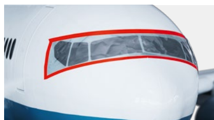
Window and window seal masking: tesa® 4308 or tesa® 4244
