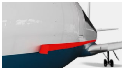
Straight-line masking : tesa® 4334 or tesa® 4104
