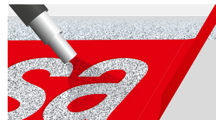
Protection during sandblasting: tesa® 4434, tesa® 4432, tesa® 4651
