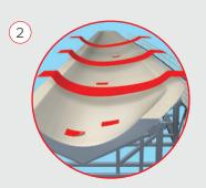
Our premium mold release tapes replace liquid release coats, when it comes to e.g. main mold repair, flat molds or mold edges. Once applied, they reduce the mold preparation time and enable shorter cycle times.
