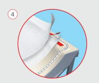
During the lay-up process our double-sided adhesive tapes are used to fix different layers to the mold or to each other. Choose from our assortment based on your requirements for adhesion, removability and temperature resistance.
