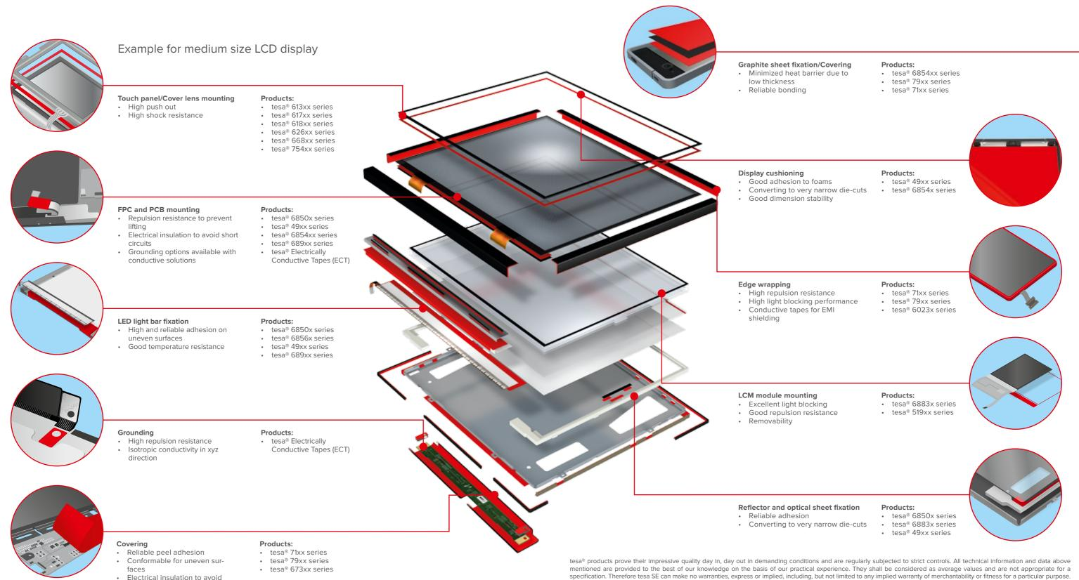
Electrical insulation to avoid short circuits
