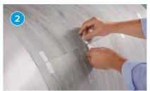
Apply splitting labels in suitable distance over entire reel width.
