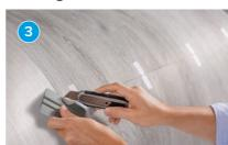
To avoid damage to the web, trim the paper's edges on both sides.
