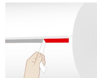
Before accelerating the reel remove the lower part of the liner – this takes a matter of seconds.
