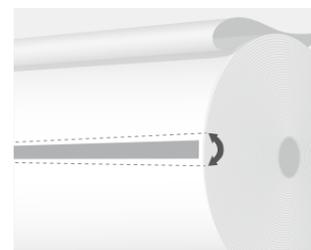
Apply the tape under the top layer of the paper roll. Then remove the upper part of the liner.
