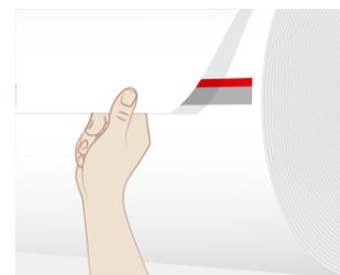
Attach the top layer onto the exposed adhesive of the tape.
