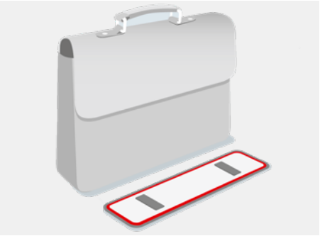
Leather mounting and lamination e.g. with tesa® 4962, tesa® 51571
