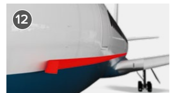
12 Straight-line masking tesa® 4334 or tesa® 4104
