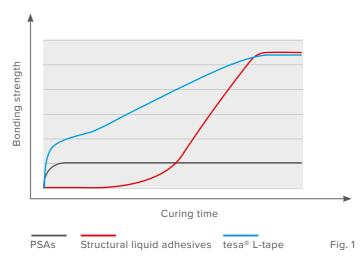
Schematic diagram of the curing time of different adhesive technologies
