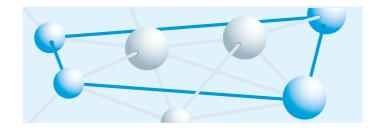
With light irradiation, the reactive acrylate forms a dense **network** with the base polymer. This gives tesa<sup>®</sup> L-tape high cohesion and provides strong and reliable bonding performance.
