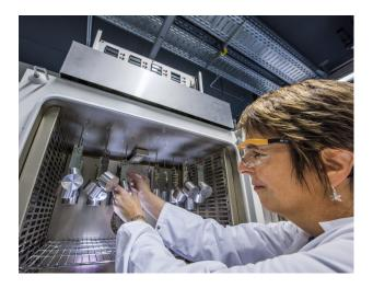
The holding power and adhesive resistance of tapes are tested using different weights. After the tapes successfully "hang in there," tesa researchers know that a particular kind of tape meets the customer's specific requirements. ("tesa SE. All rights reserved.)
