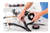
The increasingly complex structure of wire harnesses and cramped quarters in the engine compartment and vehicle interior are a major challenge for manufacturers of wire harnesses. tesa Automotive offers an extensive range of products for wire harnessing, consisting of fabric, nonwoven fabric, and film backings with high-quality adhesives. (\*\*etsa SE. All rights reserved.)
