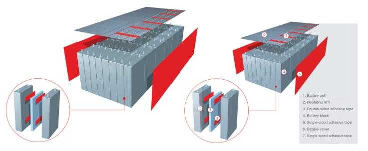
Each battery cell generates heat and electrical voltage that needs to be shielded. Double-sided adhesive tape and a special film are used to connect the cells with each other and insulate them so that no power surges, known as "overvoltage," can occur. The battery block is wrapped in non-flammable products from the tesa product range.
