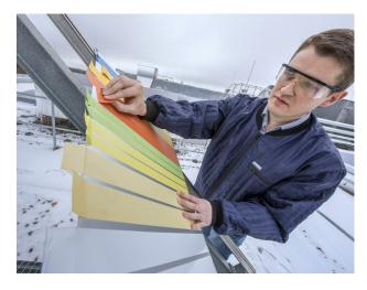
There is a weathering unit on the roof of the new tesa building. Individual strips of tape or larger items, such as entire solar panels with adhesive bonding in place, can be subjected to practical testing under real-world weather conditions here.
