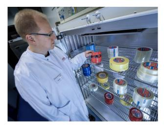
The application technology team puts products to the test. A heat chamber is used to simulate the aging process in tapes, for example. This method speeds up time so the effects can be seen in just a short period. (\*\*etsa SE. All rights reserved.)
