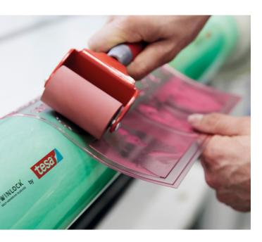
The concept of tesa Twinlock® is simple: a self-adhesive and compressible sleeve to mount your flexo printing plates.
