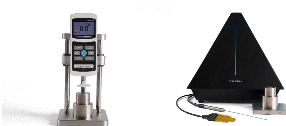
Figure 3. Left) MTPS mounted in the Compression Test Accessory (CTA). Right) C-Therm's Trident thermal conductivity instrument.
