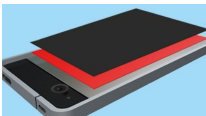
Cushioning material lamination
