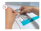
To avoid damage to the web, trim the paper's edges on both sides of tesa® EasySplice to avoid air pockets underneath the unsecured edges.
