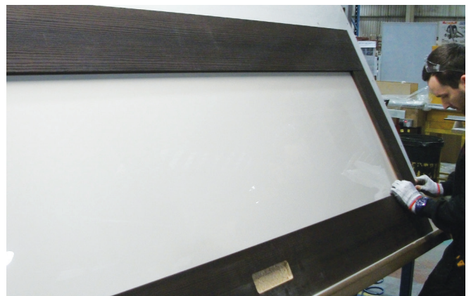
Door panels being located
