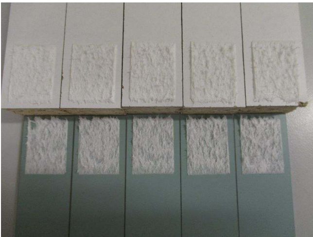
Pic. 3: rupture pattern after loading with 4.2 N/cm² (load stage 9%)
