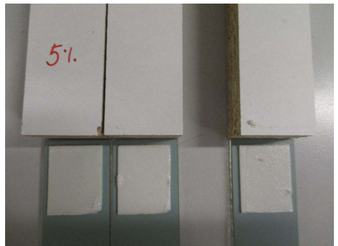
Pic. 4: rupture pattern after loading with 2.1 N/cm² (load stage 5%)
