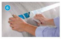
Carefully remove the liner in the direction of the splitting labels. Ready to splice!
