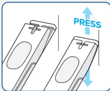
When pressing, make sure that the line at the top of the *pressing tool* closes, then you are pressing hard enough.
