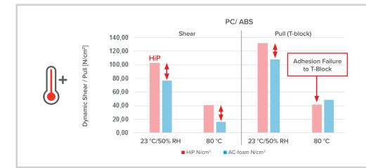
tesa<sup>®</sup> HiP shows a reliable bond in the temperature range from -30°C to 100°C, required for interior applications.
