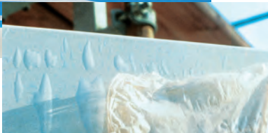
Application of self-adhesive protective film on anodised aluminium surface not free of bubbles and wrinkles
