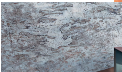
Surface change due to condensation on zinc sheet
