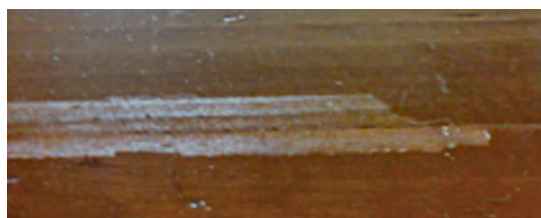
Stripping of the imitation wood; high risk with standard masking tape if removed when wet. No damage with tesa Precision Mask® 4333 Sensitive
