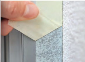
Adhesive residues on anodised aluminium
