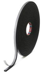
Soft grade skinned PVC/Nitrile closed cell single sided foam tape 9mm thick (black)
