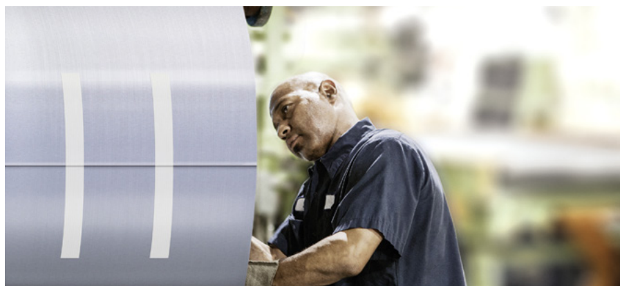
tesa strapping tape used for end tabbing on aluminium coil
