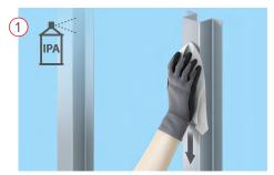
Clean substructure in one direction with appropriate solvents using a lint-free cloth.
