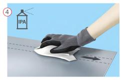
Clean panel in (one direction) with appropriate solvents using a lint-free cloth. Allow solvents to evaporate.
