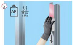
Shake the tesa® Adhesion Promoter can before opening. Apply tesa® Adhesion Promoter with a tool. Allow solvent to evaporate. Always close the can after usage.
