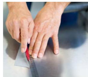
Put the tape on a flat surface and cut it diagonally from the end of the roll to the marked point of the tape.
