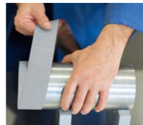
Keep on wrapping the roller with the tape at even angles, leaving no gaps in between the layers.
