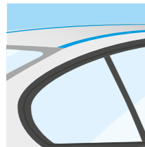
Roof ditch trim
