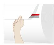
Attach the top layer onto the exposed adhesive of the tape.
