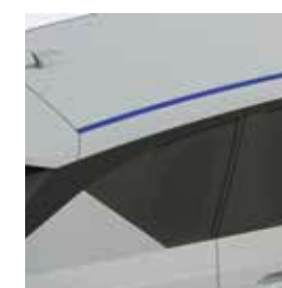
Roof ditch trim
